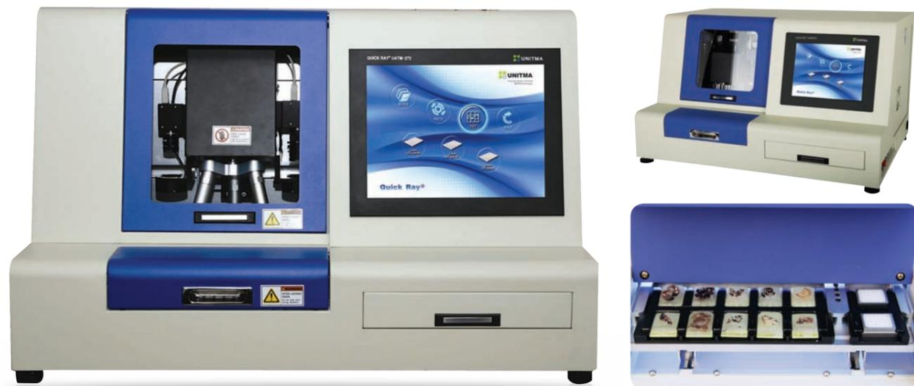
Quick Ray Master is an automated tissue microarrayer running by the built-in PC. The instrument extracts the sample tissues from the donor blocks and delivers the extracted sample tissues into the correspondent hole of the premade recipient block automatically.
